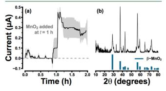
Figure 5. (a) Addition of  $MnO_2$  to one-half-cell at t=1 h resulted in oxidation of lead in the other, as indicated by an increase in the magnitude of galvanic current between the two lead electrodes. The black line denotes the mean and the shaded region spans the range of duplicate tests; the current signal was smoothed with a 200-point moving average. (Raw data with computed detection limits are provided in Figure S7.) (b)  $MnO_2$  was identified as pyrolusite (β- $MnO_2$ ) by XRD.
